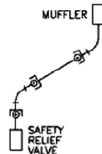
Figure 9: Three ball joints installed in safety relief valve piping.
